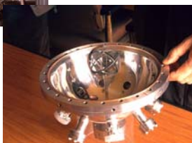
The Inertial Electrostatic Confinement Fusion Devices used as Portable Neutron Sources (Institute of Advanced Energy Kyoto)
